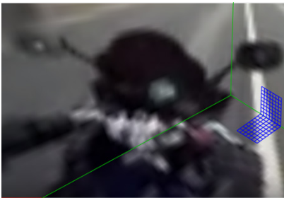
Figure 6. Example of viewport extracted for compressed cube-map panorama: discontinuities between the cube faces in the panoramic arrangement (highlighted by green lines) may cause wireframe cube and underlying image sampling domain (highlighted by blue grids) to be visible.
