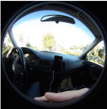
Figure 1. Example of optical distortions: image captured with fish-eye lens.
