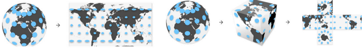
Figure 3. Example of map projections (equirectangular on the left, cube map on the right) and related warping distortions: blue circles on the spherical surface are mapped to ellipses with varying axis lengths on the plane.
